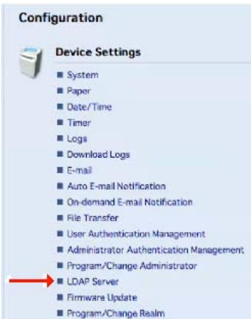
Once we are on the *LDAP Server* settings page we hope to find LDAP services configured and enabled. In this example we see that ACMECD01 is listed as the authenticating LDAP server (Figure 5). From here it's as simple as selecting the LDAP setting you wish to modify and clicking on *Change*.
